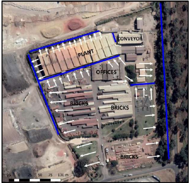
Figure 9: Existing Storm Water Structures
