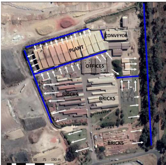
Figure 5:15: Existing Storm Water Structures (MVD Kalahari Consulting, 2024)
